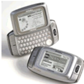
The Danger Hiptop is a PDA, a mobile phone, and an MP3 player with the look and feel of a digital camera.
